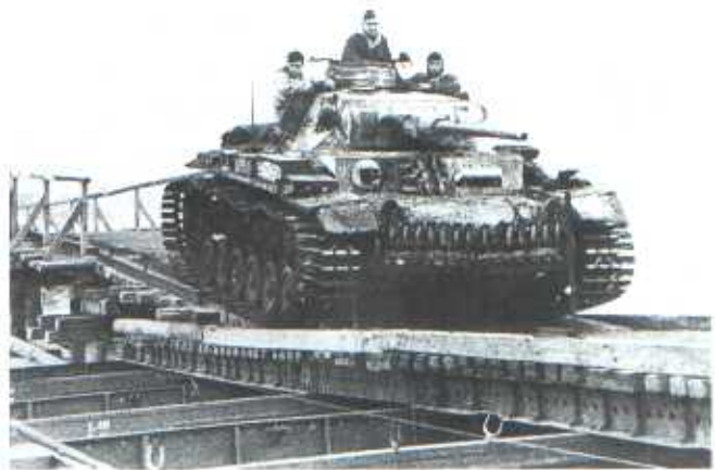
PzKpfw III (Sd Kfz 141) Ausf. J z 23. DPanc, Stalingrad, 1942 rok. PzKpfw III (Sd Kfz 141) Ausf. J of the 23. Panzer Division, Stalingrad, 1942. Note 'Ostkette' tracks [Tank Museum]
